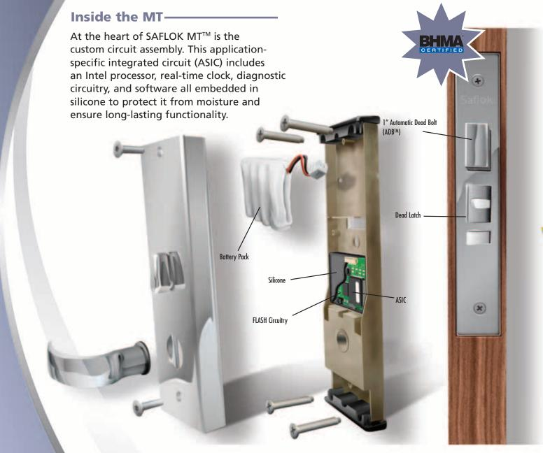
The non-volatile FLASH circuitry stores over a year's worth of lock data (or up to 5,900 entries) providing detailed audit-trail information such as date and time of the entry as well as the ID code of the employee or guest using the keycard.
